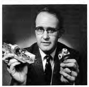
PROTOTYPE of a cold cathode gauge suitable for use in a small sounding rocket and a manufactured model (right) are held by inventor Robert Woods (5235).
